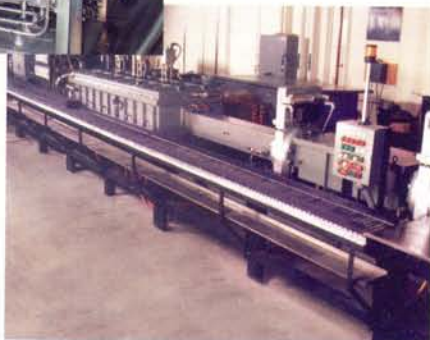
High temperature (2300°C cold-wall) debind and sinter pusher for ceramics
