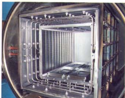
Hydrogen furnace (1600°C) with a custom molybdenum retort
