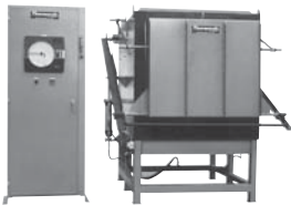
Front Loading Box Furnace with pneumatic, vertical lift door
