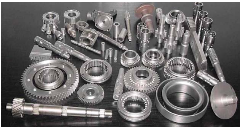
Fig. 3. Family of aerospace, automotive and industrial components illustrating the versatility of low-pressure vacuum carburizing
