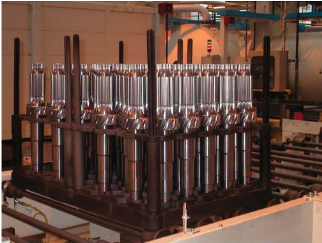
Fig. 4. Heavy-duty truck shafts low-pressure vacuum carburized and oil quenched
