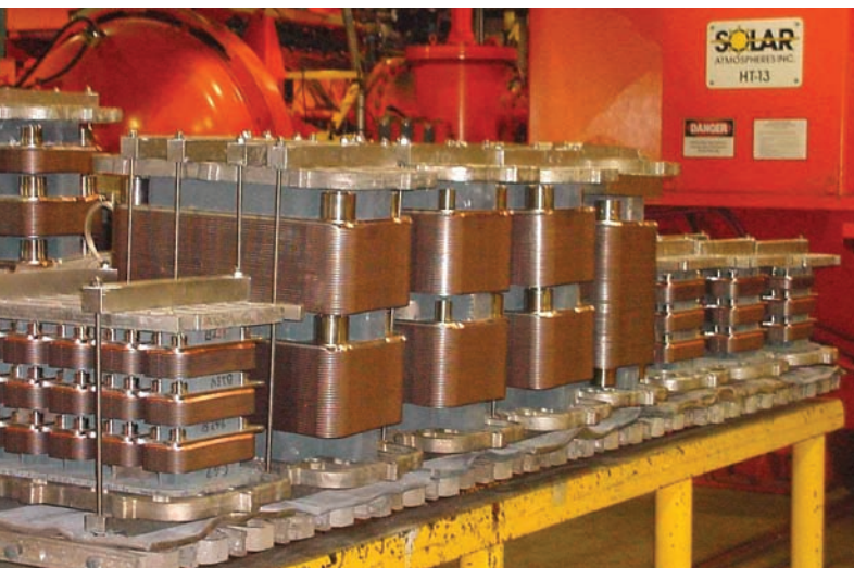
Load of flat-plate heat exchangers ready for brazing at 5 torr nitrogen partial pressure at 1120°C. Photo courtesy of Solar Atmospheres Inc.
