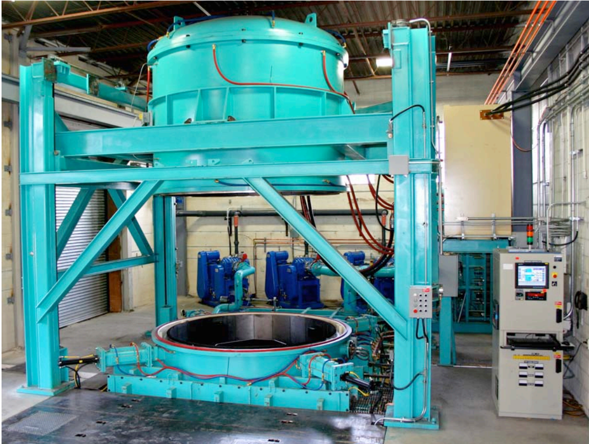
Figure 6 Typical Vertical Vacuum Oil Quench Furnace (Photograph Courtesy of Vac-Aero International)
