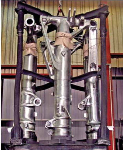
Fig. 8. Landing-gear load being assembled for hardening and oil quenching in a vertical vacuum furnace (Photograph courtesy of Vac-Aero International)
