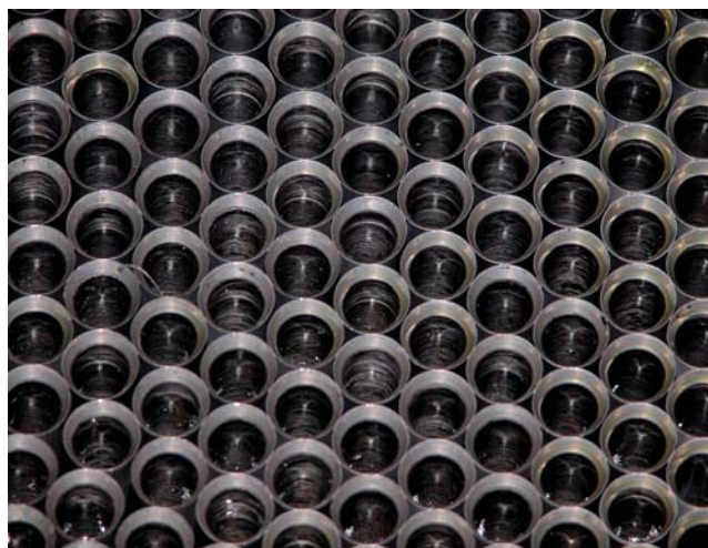
Fig. 7. Die-cutting punches after oil quenching in a horizontal batch vacuum furnace
