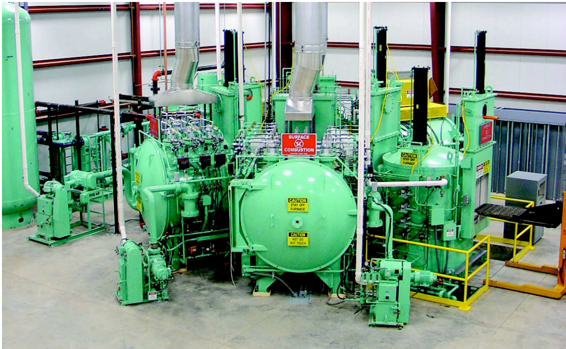
Figure 13 Multi-Chamber Vacuum Carburizing System with Four (4) Heating Chambers, One (1) Oil Quench Chamber, & One (1) High Pressure Gas Quench (Courtesy MMS Thermal, Davenport, IA)
