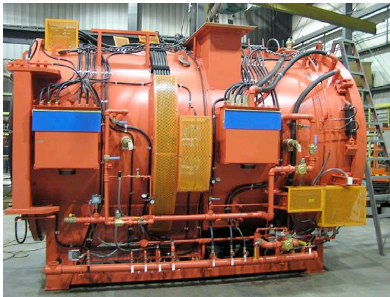
Figure 11 Two Chamber Gas Quench Multi-Chamber Vacuum Furnace (Courtesy of Surface Combustion)
